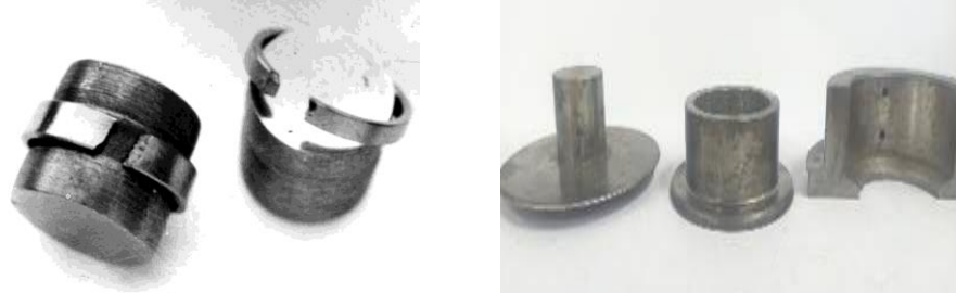
Fig. 4. Type of ring samples brought to destruction by distribution on deformable mandrels
