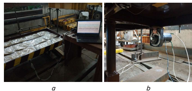
Fig. 2. Experimental setup: a – general view; b – vibration exciter with an unbalanced mass position sensor
