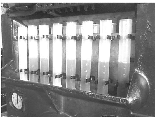
**Fig. 10.** The measurement of the cycle biofuels supply at the KI-921-M booth
