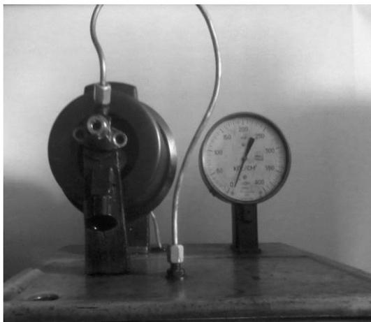
**Fig. 9.** The measurement of the fuel injection angle at the KI-22203 booth ( $L=92$  mm)
