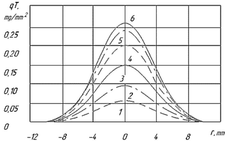
**Fig. 4.** Changing the dispersion of spraying  $q_T$  along the radius of the jet  $r$  at a distance of  $L = 50$  mm from a spray hole with a diameter  $d = 0.25$  mm at injection pressure  $r_{vp} = 1.85$  MPa and cycle feed  $g_{is} = 8$  mg at different points in time  $\tau$  from the beginning filling: 1- $\tau = 1,026$ ; 2-1,282; 3-1,538; 4-1,795; 5- 2.05; 6-2,30.
