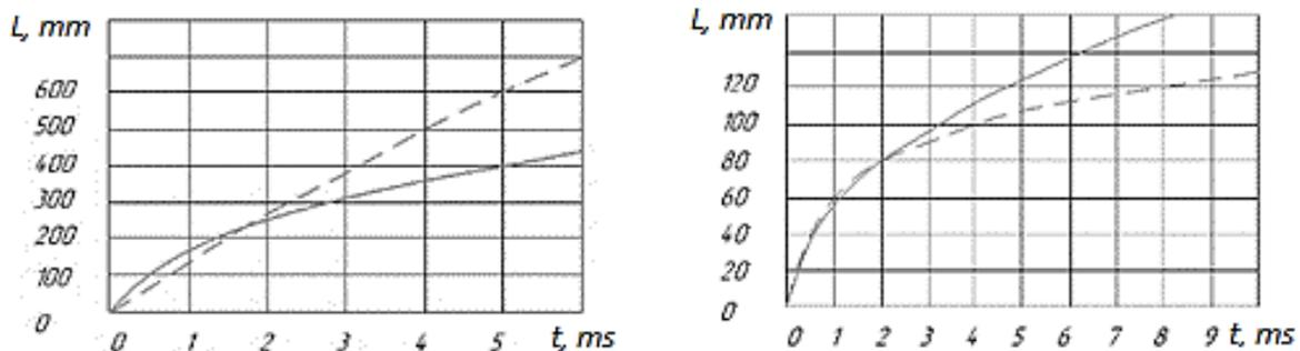
**Fig. 1.** Estimated values of the fuel jet length L: solid line - by the method of A. Lishevsky; intermittent - MADI technique [28], a -  $p_{inj} = 26$  MPa,  $p = 0,1$  MPa,  $d = 0,54$  mm,  $\delta$  -  $p_{inj} = 26$  MPa,  $p = 1,1$  MPa,  $d = 0,23$  mm.
