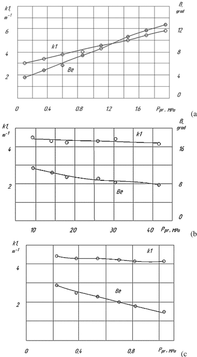
**Fig. 8.** Dependences of the coefficient  $k_1$  and the angle  $\beta_e$  on the counter pressure  $p_{pr}$  (a) and the spray pressure  $p_p$  (b) of the spray hole diameter  $d_p$  (c)
