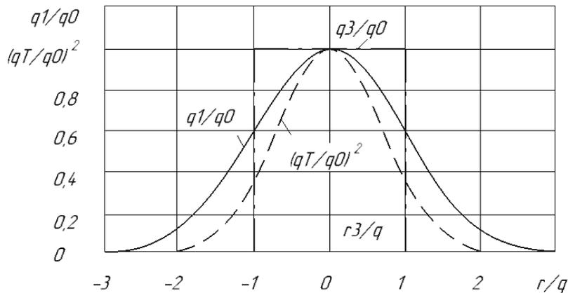
**Fig. 5.** Characteristic of the change of irrigation density  $q_T$ , square of irrigation density  $q_T^2$  and equivalent density  $q_e$  related to axial density  $q_0$ .
