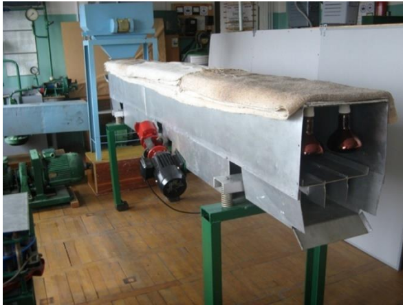
Figure 1. Photo of the experimental vibrating tray infrared dryer
