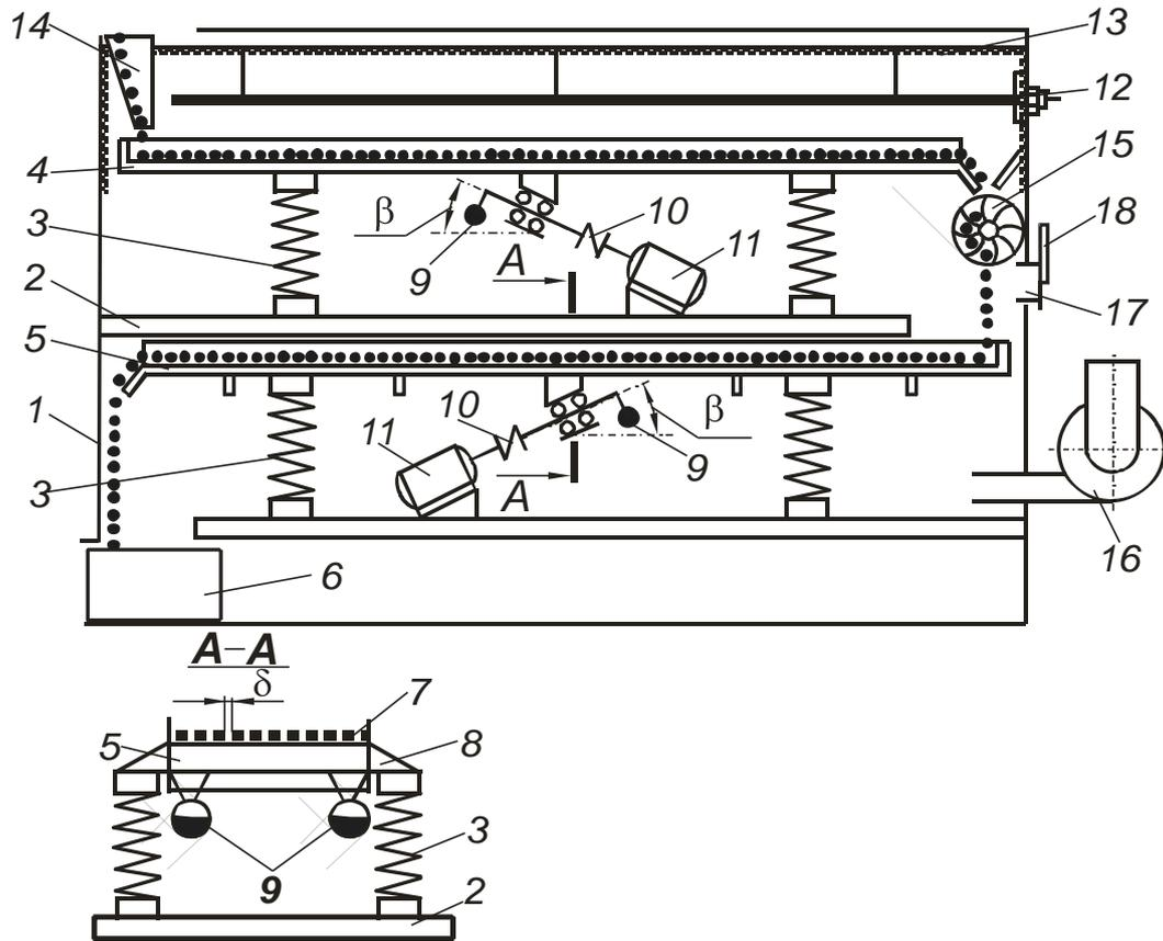
**Fig. 1 - Scheme of laboratory infrared monochrome vibration dryer**
