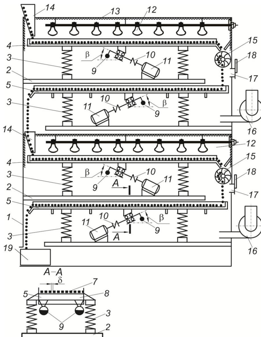
**Fig. 6 - Principal scheme of vibration monolayer lot dryer**
