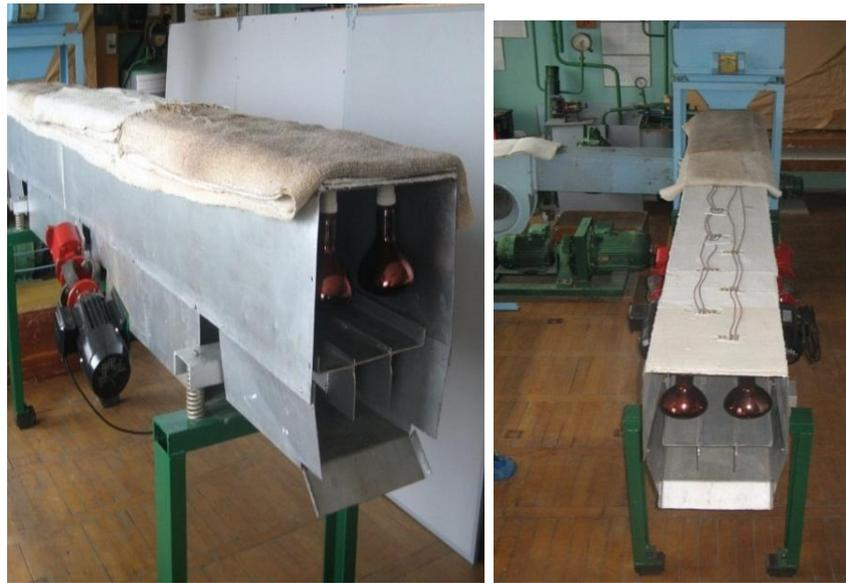
**Fig. 2 - Photo of experimental vibrotray infrared dryer**
