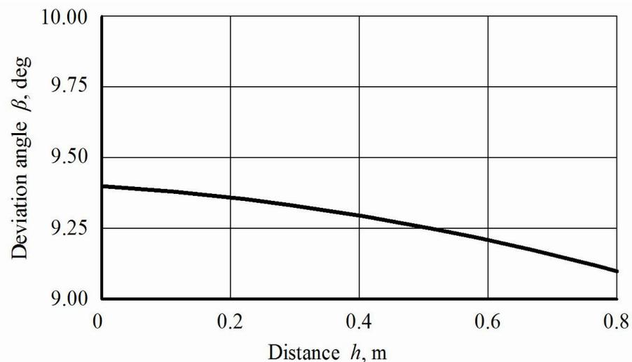
Fig. 6. Dependence of deviation angle  $\beta$  of trailed swath header upon value of left-side offset (drag)  $h$  of wheel at speed  $V_o$  of aggregate 2.8 m·s<sup>-1</sup> (at  $M = 0$ )
