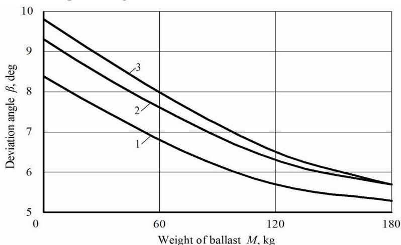
Fig. 4. Dependence of deviation angle  $\beta$  of swath header in horizontal plane upon ballasting mass  $M$  of its left supporting wheel, offset by  $0.4 \text{ m}$ , and different speeds  $V_o$  of operating movement of aggregate: 1 –  $2.1 \text{ m}\cdot\text{s}^{-1}$ ; 2 –  $2.8 \text{ m}\cdot\text{s}^{-1}$ ; 3 –  $3.7 \text{ m}\cdot\text{s}^{-1}$
