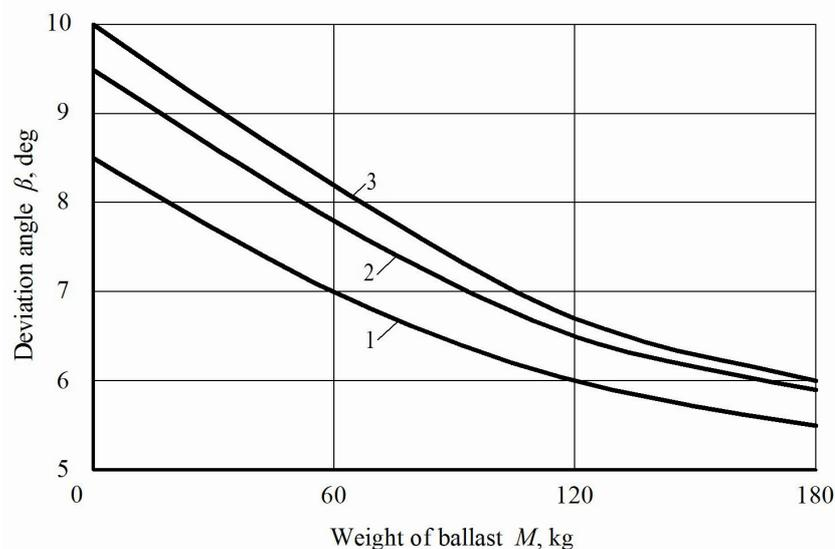
Fig. 3. Dependence of deviation angle  $\beta$  of trailed swath header in horizontal plane upon value of additional load (ballasting mass)  $M$  on left supporting wheel at various speeds  $V_o$  of operating movement of aggregate: 1 –  $2.1 \text{ m}\cdot\text{s}^{-1}$ ; 2 –  $2.8 \text{ m}\cdot\text{s}^{-1}$ ; 3 –  $3.7 \text{ m}\cdot\text{s}^{-1}$
