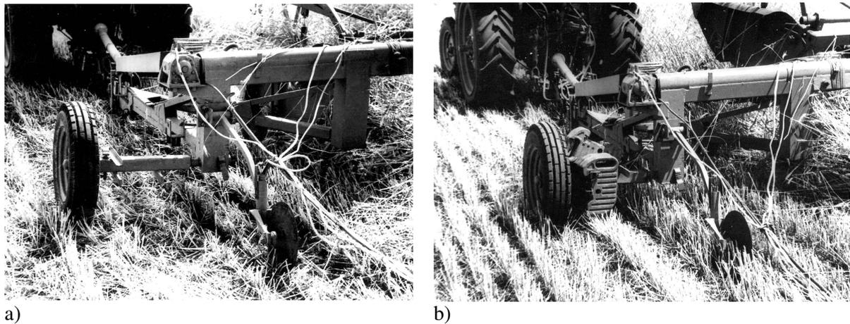
Fig. 2. Experimental variant with arrangement of left supporting wheel of trailed swath header at distance (a) and with additional load (additional vertical mass on the bracket of the left wheel) – (b)
