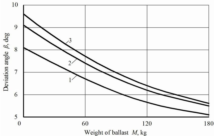
Fig. 5. Dependence of deviation angle  $\beta$  of swath header in horizontal plane on value of additional vertical mass of left supporting wheel arranged at distance of 0.8 m from trailing device and on various operating speeds: 1 – 2.1 m·s<sup>-1</sup>; 2 – 2.8 m·s<sup>-1</sup>; 3 – 3.7 m·s<sup>-1</sup>
