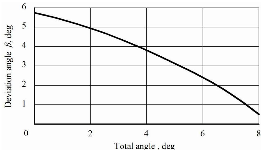
Fig. 7. Total impact of turning angles of left ( $\alpha_1$ ) and both right ( $\alpha_2$ ) support wheels of trailed swath header upon its deviation angle  $\beta$  in horizontal plane, at speed  $V_o$  of its operating movement  $3.7 \text{ m}\cdot\text{s}^{-1}$
